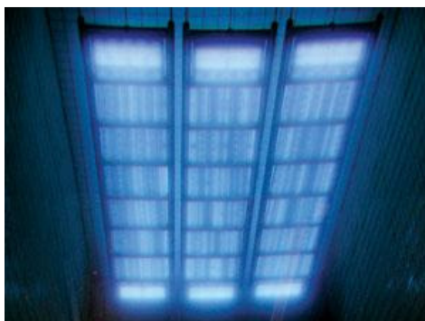
Figure 1. Gamma rays are generated from Cobalt-60 sources (shown above). Photo courtesy of STERIS Isomedix Services.
