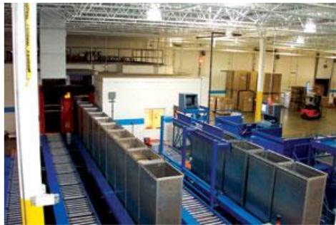
Figure 2. Totes entering an irradiation chamber according to a predetermined loading pattern. Photo courtesy of STERIS Isomedix Services.
